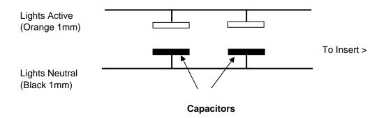
Total capacitance required per insert will be the number of fluorescent lights multiplied by;
