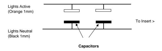
Total capacitance required per insert will be the number of fluorescent lights multiplied by;
